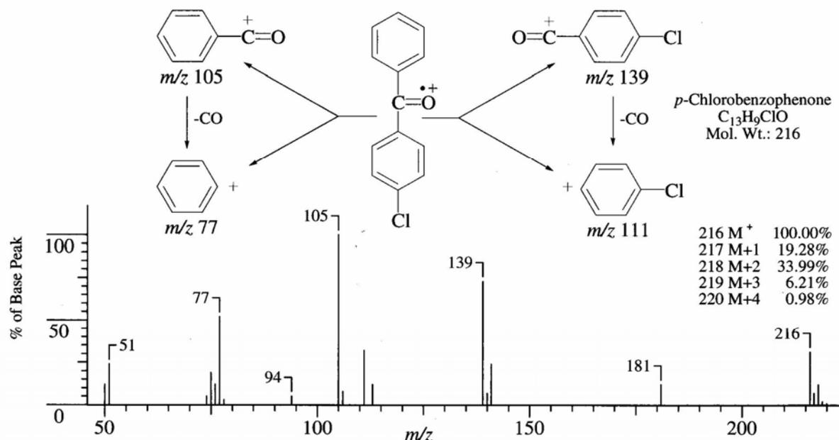
FIGURE 1.23 EI mass spectrum of p-chlorobenzophenone.
