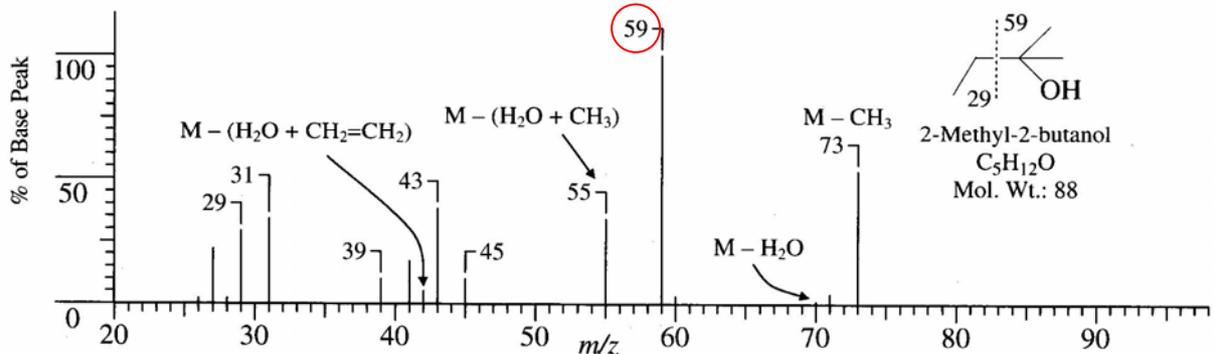
FIGURE 1.18 EI mass spectra of isomeric pentanols.
