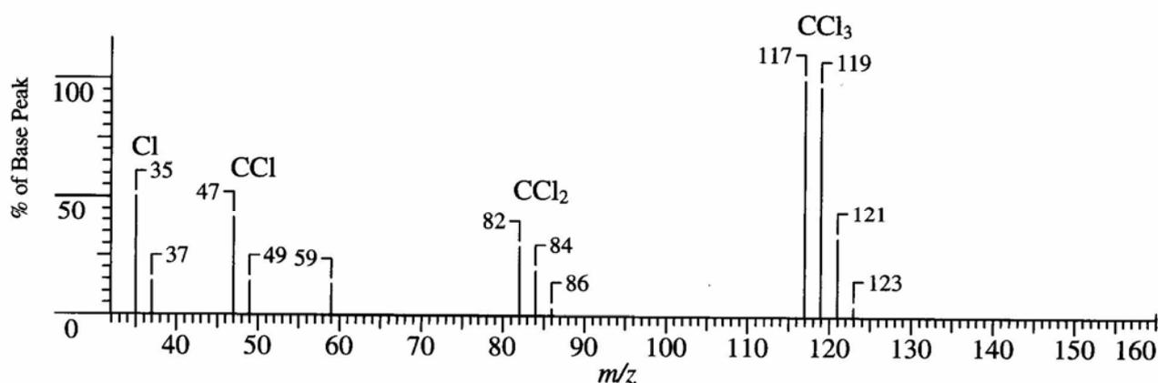
**FIGURE 1.30** EI mass spectrum of carbon tetrachloride ( $\text{CCl}_4$ ).
