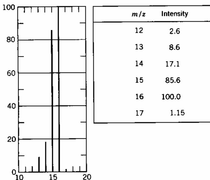
**Figure 8.2** Mass spectrum of CH<sub>4</sub> in both bar graph and tabular form.
