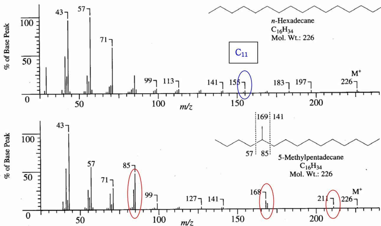
**FIGURE 1.14** EI mass spectra of isomeric  $\text{C}_{16}$  hydrocarbons.
