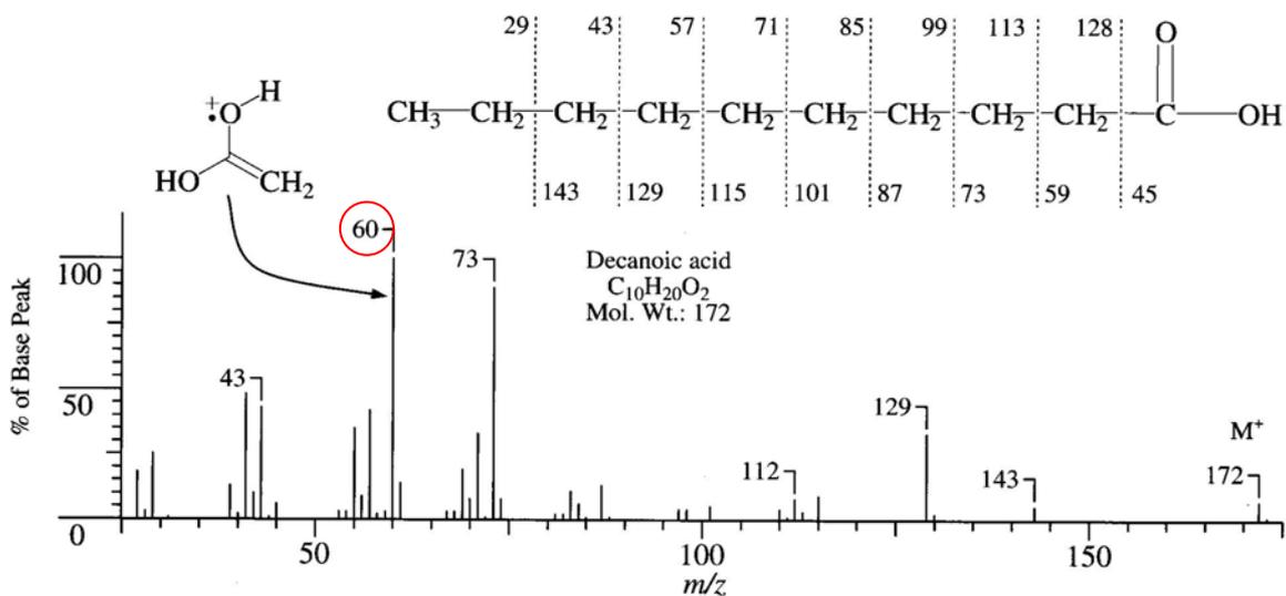
FIGURE 1.25 EI mass spectrum of decanoic acid.
