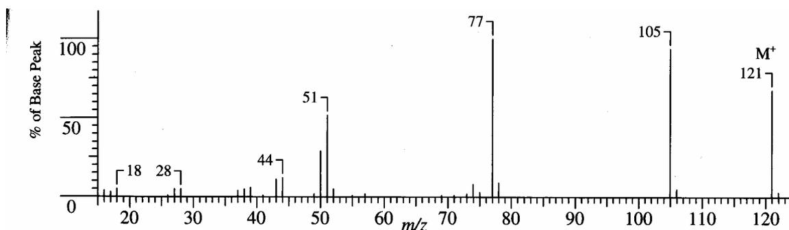
**FIGURE 1.1** The EI mass spectrum of benzamide above which is a fragmentation pathway to explain some of the important ions.
