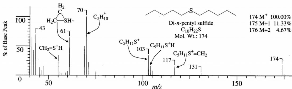
**FIGURE 1.28** EI mass spectrum of di-*n*-pentyl sulfide.
