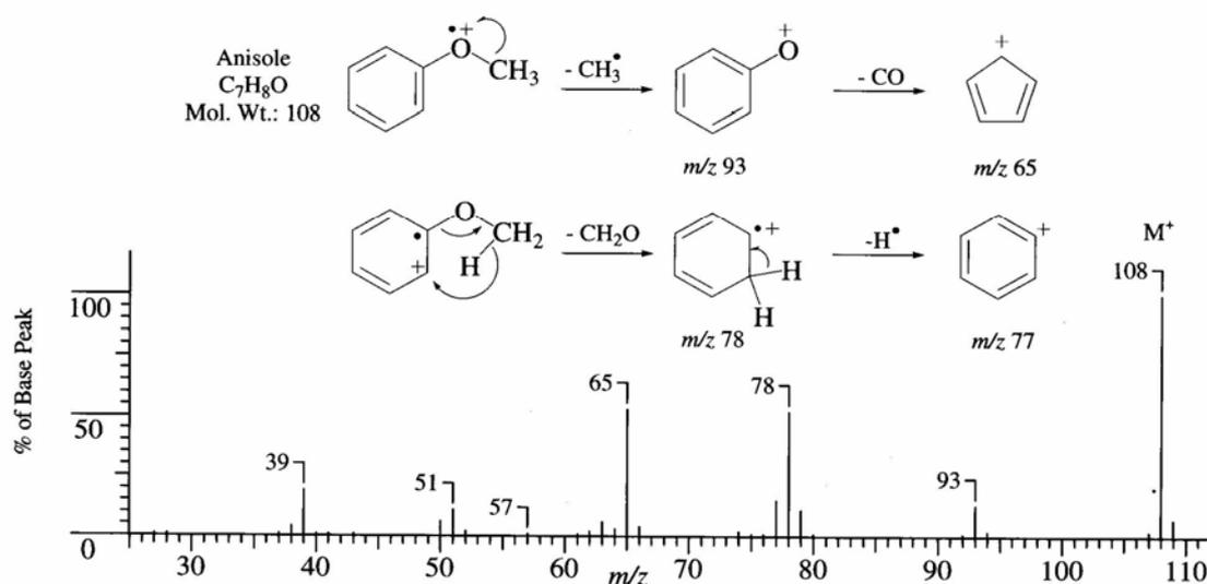
FIGURE 1.21 EI mass spectrum of anisole.
